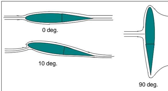
The sketches at 0 degrees and 90 degrees seem quite reasonable. Clearly, the flow over a symmetrical airfoil at 0 degrees will divide symmetrically at the nose and continue symmetrically to the trailing edge with no lift generated. At 90 degrees, the airfoil is like a flat plate at right angles to the stream direction, and air will flow around both sides, probably separating as it tries to go round the edges.
