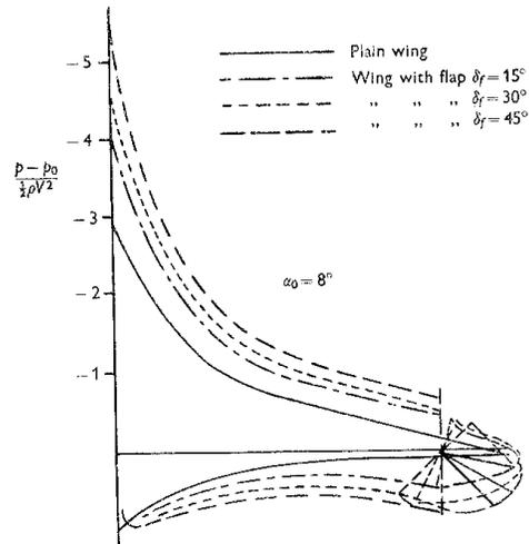
Fig. 14-2. NACA 23012 section and 0.2c plain flap. Change in pressure distribution due to flap deflection.
