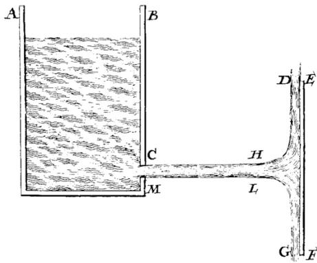
Fig. 4-3. Liquid jet flowing from a vessel and impinging onto a flat plate. From D. Bernoulli, *Hydrodynamica* (Strasbourg, 1738), fig. 84.
