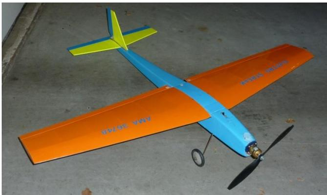
The other is a semi-free flight Rascal. I fell for that nice elliptical wing with moderate dihedral, and no ailerons, and felt that I could kick back and watch it fly itself – or almost!
