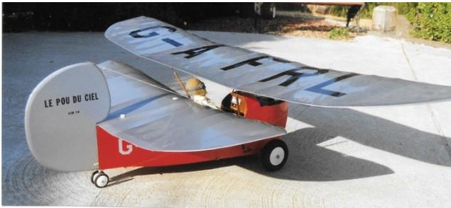
This is a 1/4 scale model of Henri Mignet's Flying Flea, or Pou du Ciel, his 14<sup>th</sup> in a series of projected home-built airplanes of the 1930's. And yes, the 66" span model flies nicely with a 0.30-sized motor.
