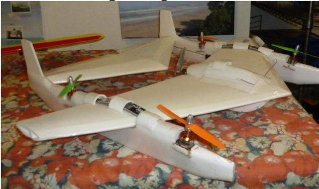
This one has the simplifying feature of having one fixed motor for conventional forward flight, and four fixed motors for vertical flight. No reports to date on flight results for this SLT (separate lift-thrust) airplane, but the avionics should be much more straightforward.
