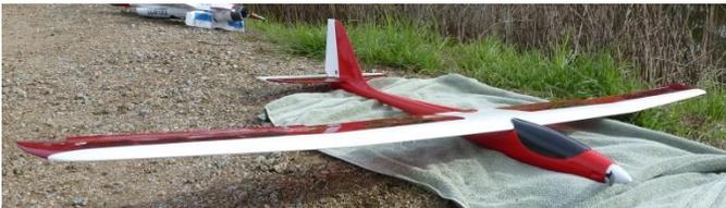
Alan Brown flew a variant of an old Electric Kaos, planned for fun-fly competition; light weight, low drag, 4S battery power and flap/aileron mixing. First flight showed the need for a bit more aileron expo, but otherwise O.K. The weight seems satisfactory at 24 ounces for 46" wingspan.
