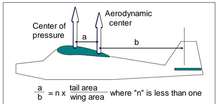
Now we'll look at the effects of distance between the wing and tail, and the wing aspect ratio. I've made some calculations to give the dimension 'a' in the figure, relative to tail arm, 'a+b', for different aspect ratios. The results are shown in the chart below.
