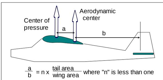
The **center of pressure** is the point where the net lift of the airplane acts and in steady level flight has to be at the same place as the c.g. of the airplane.
