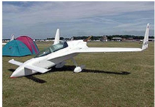
Note that the forward, canard surface is of a high aspect ratio, and one of the claims for the aircraft is that it is unstallable. Burt understands the high aspect ratio canard story very well. He's a good aerodynamicist!
