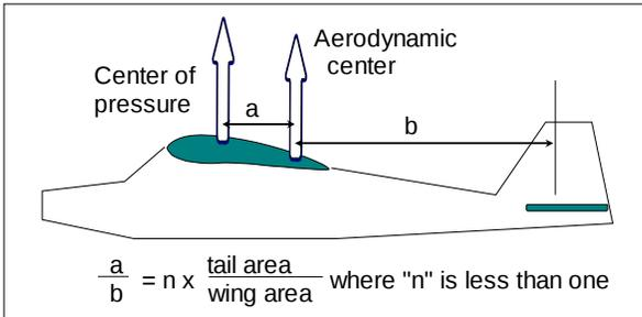
Now we'll look at the effects of distance between the wing and tail, and the wing aspect ratio. I've made some calculations, which I must admit were a bit more tedious than I expected they would be, to give the dimension 'a' in the figure on the left, relative to tail arm, 'a+b', for different aspect ratios. The results are shown in the next chart. I'll try to explain why they come out the way they do.
