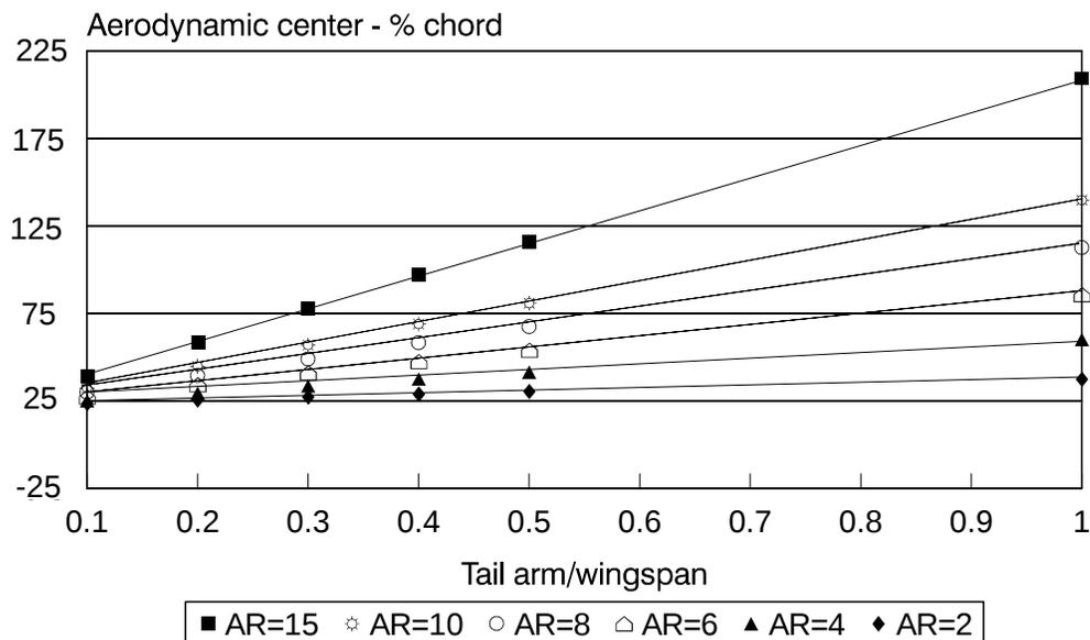
First, note that when the aerodynamic center position is greater than 100%, it is behind the trailing edge of the wing. This happens fairly readily for a high aspect ratio airplane, especially one with a long moment arm. Free flight competition models often fall into this category and are often balanced fairly close to the trailing edge in order to get the most effectiveness out of the tail. Note that as we
